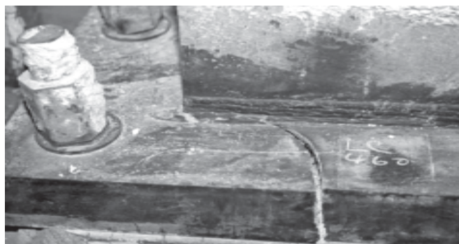
Figure 28 —A 4-inch-thick steel plate supporting the base of a column at the Oviatt Library at CSU Northridge fractured in the 1994 earthquake.
